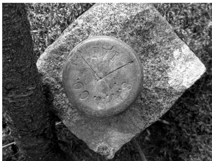
Granite post knocked over with copper disk coming out. SHR-3 FOUND · 7 Jul 2025
